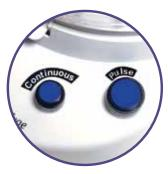
FlexiFuge can be operated in continuous mode or pulsed for rapid centrifugation
