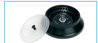
Item: Z216-6405 64 x 0.5ml Angle Rotor (40°/55°) Max Speed: 13,500 rpm / 16,298 x g* Accel: 16 sec. / Decel: 17 sec.
