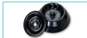
Item: Z216-1205 12 x 5ml (45°) Hermetically Sealed Max Speed: 14,500 rpm / 19,978 x g Accel: 24 sec. / Decel: 17 sec.
