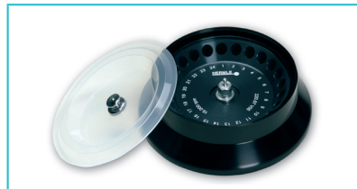
Item: Z216-2420 24 x 1.5/2.0ml Angle Rotor (45°) Max Speed: 15,000 rpm / 21,379 x g Accel: 21 sec. / Decel: 18 sec.
